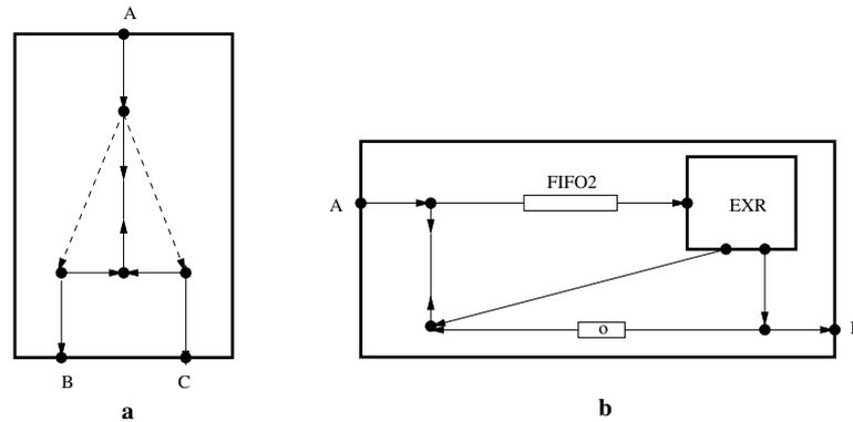
Fig. 2. Exclusive router and shift-lossy FIFO1 channel
